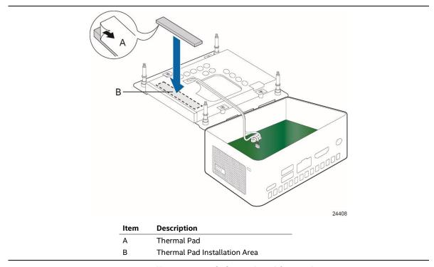
Figure 21. Installation area of Thermal Pad for Intel NUC Kit NUC8i3BEH/NUC8i5BEH/NUC8i7BEH
