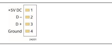
Figure 14. Connection Diagram for the Internal USB 2.0 Single-Port Header (1.25 mm Pitch)
