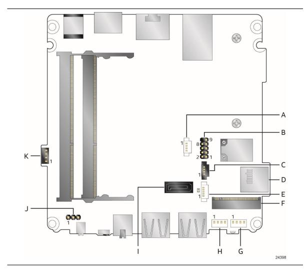
Figure 12. Connectors and Headers (Bottom)
