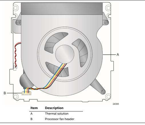
Figure 7. Thermal Solution and Fan Header
