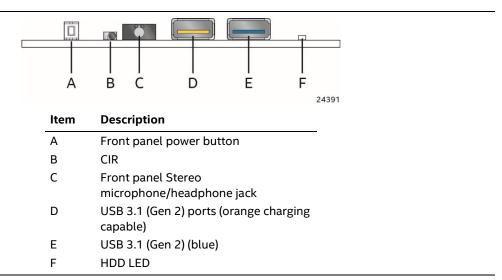
Figure 9. Front Panel Connectors
