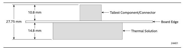
Figure 18. Board Height Dimensions
