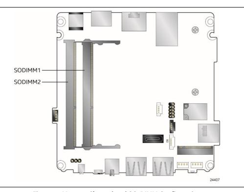
Figure 4. Memory Channel and SO-DIMM Configuration
