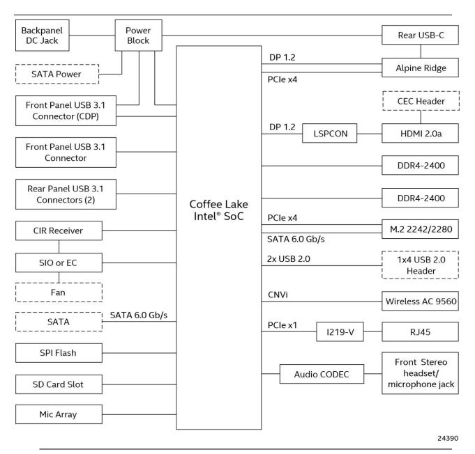
Figure 3. Block Diagram
