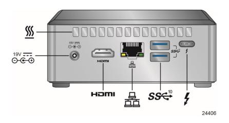
Figure 24. Intel NUC Kit NUC8i3BEH/NUC8i5BEH/NUC8i7BEH Features – Rear
