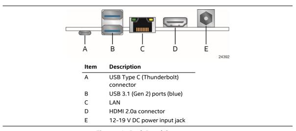
Figure 10. Back Panel Connectors
