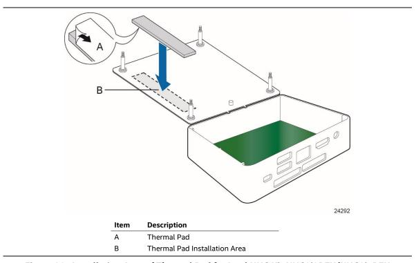
Figure 20. Installation Area of Thermal Pad for Intel NUC Kit NUC8i3BEK/NUC8i5BEK
