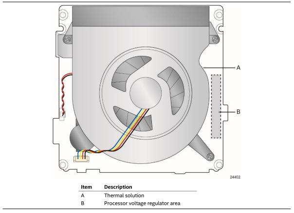
Figure 19. Localized High Temperature Zones
