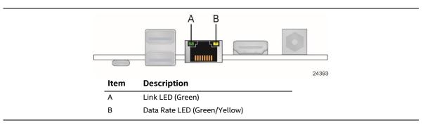
Figure 6. LAN Connector LED Locations
