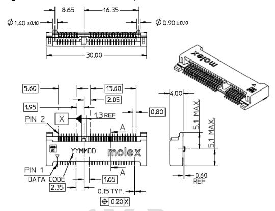
Figure 6-2 Dimensions of the Mini PCI Express connector
