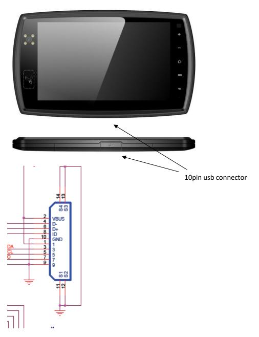
pls see the above schematics of our USB connector in our PND, it is 10 pin connector. Pin 4 and 6 can be used for USB or TTL serial interface (Rx/Tx) and Pin 8 is ID pin which is used to distinguish for USB or serial interface.
